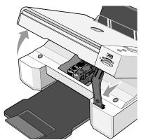
The ink cartridge carrier moves and stops at the loading position unless the printer is busy.
